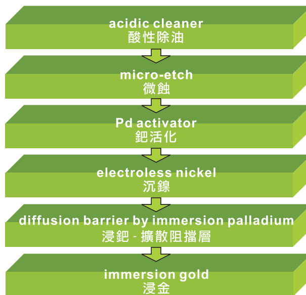
Figure 3: Process sequence of the electroless nickel/immersion palladium/immersion gold process (ENIPIG) 圖 3: 流程次序，沉鎳/浸鈀/浸金 流程 (ENIPIG)
